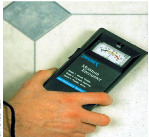
Figure 12. Moisture detectors can help pinpoint areas of excessive moisture hidden inside walls.
